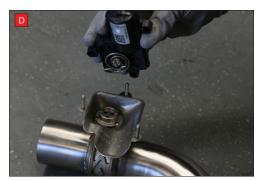
now be able to see the torsion spring (This must stay on the electronic valve motor to work with Scorpion Exhaust).
